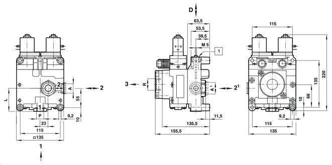
$\boxed{1}$  Flange surface for pressure switch and failure indicator unit
